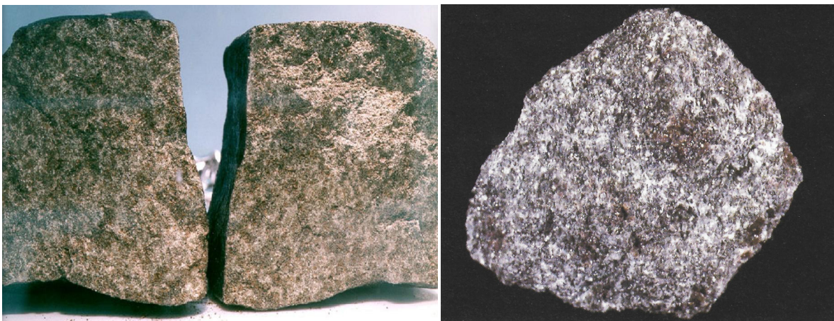
Fig. 3. The Nakhla meteorite is the prototype of the nakhlite Martian meteorites. Some 40 fragments of the Nakhla meteorite totaling 40kg were seen to fall as a shower in the hamlets surrounding the village of El-Nakhla, El-Bahariya in Egypt (near Alexandria) on June 28th, 1911, at 9:00 a.m. (a) Inside surfaces after breaking in 1998. (Public domain photo courtesy of NASA.) (b) This is a 4.02 g sample from one of the forty fragments. This specimen is 19 mm across and is housed in the Institute of Meteoritics, University of New Mexico (after Norton 2002).
