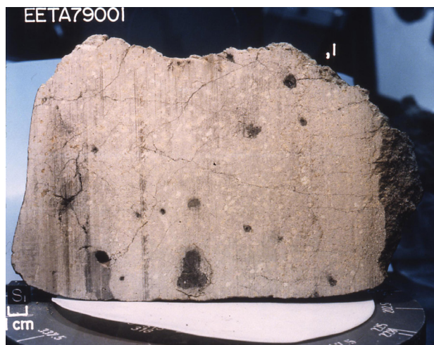
Fig. 8. End cut after first saw cut of EETA79001 Martian meteorite. It was found on January 13, 1980, in the Elephant Moraine area of Antarctica and weighed 7.9 kg. Sawing was done with a steel band saw without any lubricant. Vertical stripes are saw marks. The cube in the lower left corner is 1 cm 3 . (Public domain photo courtesy of NASA.)
