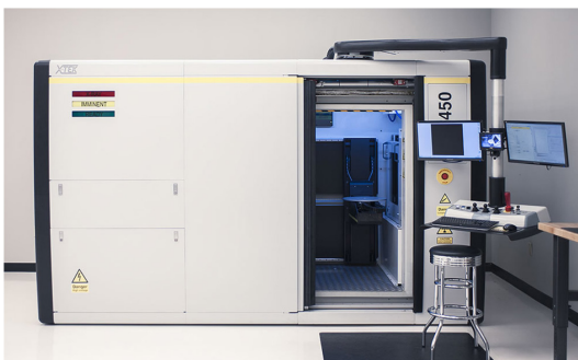
Fig. 2. The Nikon XT H 450 scanner that was used to create the CT scans. Photo courtesy of Answers in Genesis.
