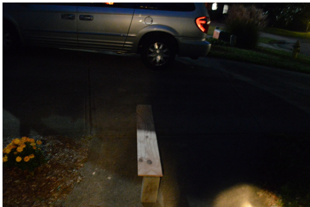
Fig. 1. The plywood board supported on bricks with half the board in moonlight and half the board in shade. The glow to the lower right is the light of a flashlight.
